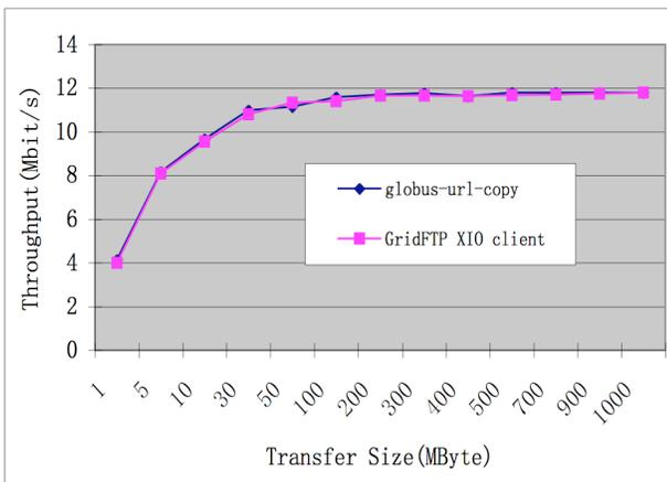
Figure 3: Comparison of performance of the XIO client with globus-url-copy over a TeraGrid network between ORNL and SDSC (72 ms round-trip time)
