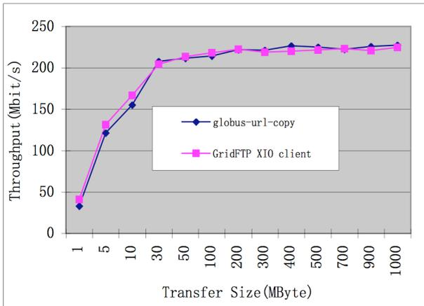
Figure 2: Comparison of performance of the GridFTP XIO client with globus-url-copy over a TeraGrid network between Argonne and NCSA (4 ms round-trip time)
