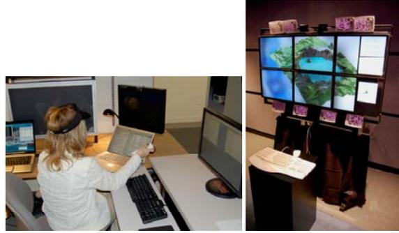
Figure 4: We deployed three autostereo systems to date at Argonne: a 30-inch personal Varrier display (left side of left image), a 17-inch active barrier display (center of left image), and a 60-inch 6-panel Varrier display (right image)
