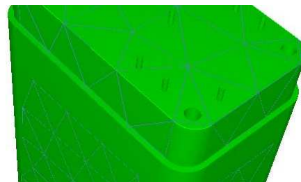
Figure 2: A part resolved to a coarse mesh size, 0.5, including appropriate amount of geometric detail.
