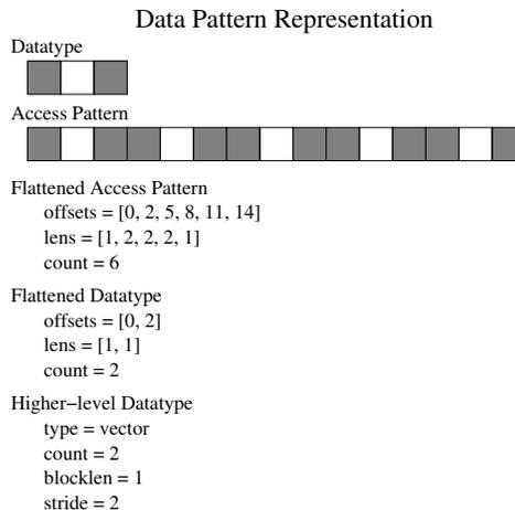
**Figure 3. While the storage size of data patterns is important, one must consider any extra processing overhead involved. With respect to just storage size, the particular pattern determines which representation is best.**
