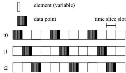
**Figure 6. One non-contiguous collective write call is made per time step. Each data point is accessed with an interleaved pattern - in this case, four processes access an element each in every data point.**
