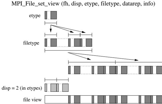
**Figure 1. File views illustrated: Filetypes are built from *etypes* which themselves may be derived datatypes. The filetype access pattern is implicitly iterated forward starting from the *disp*. An actual count for the filetype is not required as it conceptually repeats forever, and the amount of I/O done is dependent on the buffer memory type and count.**
