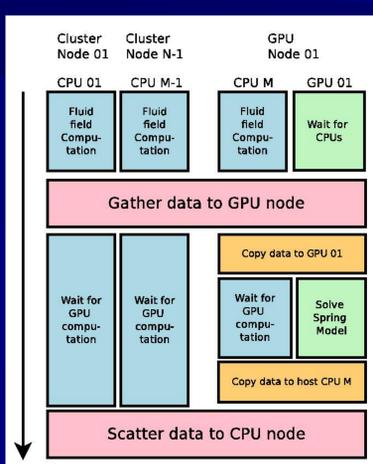
The right figure illustrates the parallelization strategy. The parallel computation of fluid field is through domain decomposition and the spring solver is accelerated by GPU computation with CUDA library. We have achieved 10 times speedup for computation of spring model.
