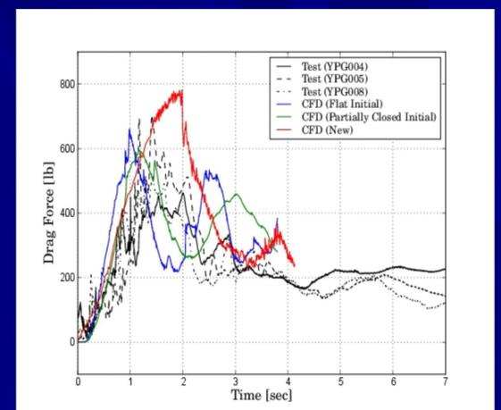
In this project, a mesoscale spring-mass model is used to mimic fabric surface motion. Through coupling with an incompressible fluid solver, the spring-mass model is applied to the simulation of the dynamic phenomenon of parachute inflation (see left figure and center figure for stress measurement). Both the tensile stiffness and the angular stiffness of the spring conform with the material's Young modulus and Poisson ratio.
