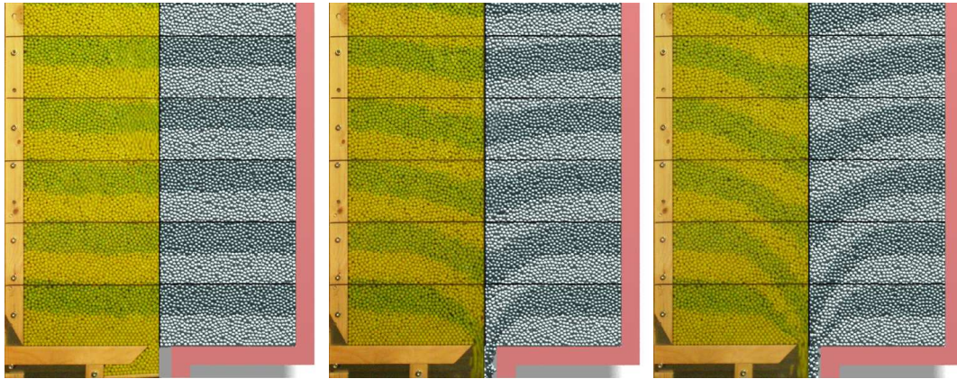
Figure 6: Comparison between experimental flow (half left of figures) and simulated flow (half right of figures) in the hopper, at time t=0 s, t=0.6 s, t=1.2 s
