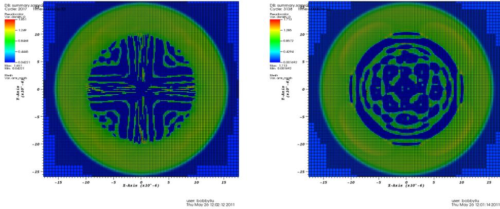
Figure 1: Results of an expanding aluminum drop without the use of surface tension model (left) and with the use of surface tension model (right). The surface tension model forms droplets while the other does not. The colorbar is shown on a linear scale from 0 to 1.7.
