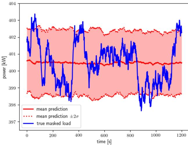
Fig. 4. Masked load (truth) and its reconstruction (prediction) through our disaggregation strategy. The predicted masked load is represented by the mean value process and  $\pm 2\sigma$  deviation. The true value is covered as close to 90% by the prediction envelope, as expected.
