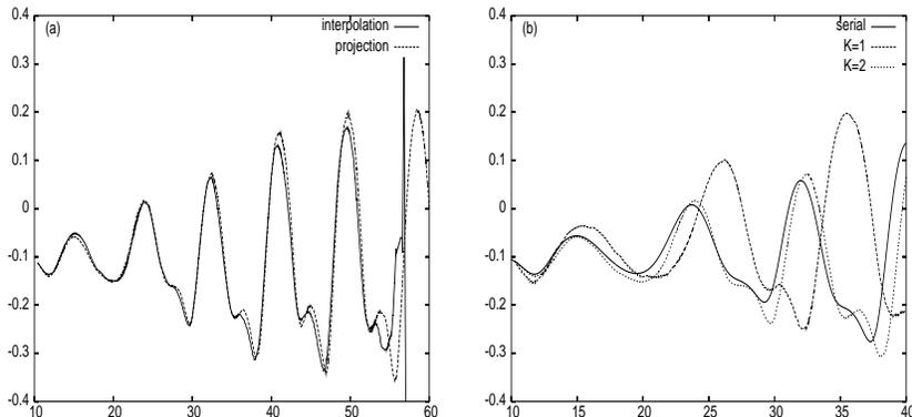
**Fig. 1.** Time history of the vertical component of the velocity at point  $(1.5, 0)$  for the parareal algorithm with coarse operator based on coarse spatial and temporal discretization. (a) Comparison of interpolation and  $L^2$  projection operators. (b) Comparison  $K = 1$ ,  $K = 2$ , and standard serial algorithms.
