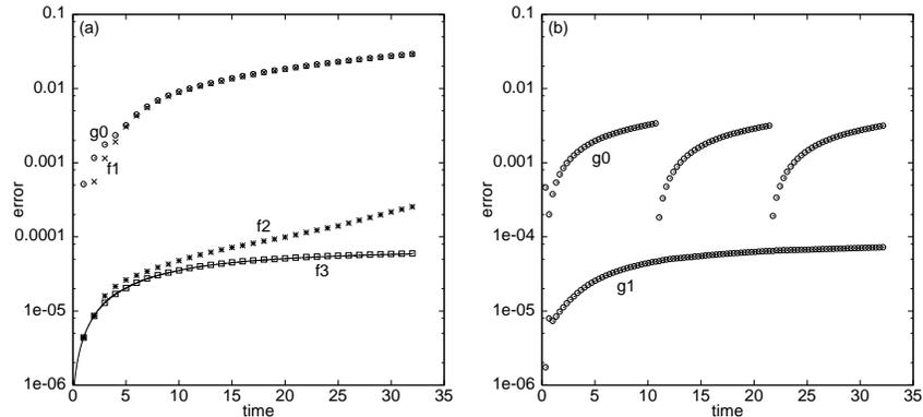
**Fig. 2.** Relative error in the  $v$ -component of the solution, versus time, for the SEM solution of the Orr-Sommerfeld test problem with  $E = 15$ ,  $M = 15$ , and  $\delta t = .005$ . (a) single partition with  $K = 3$ , (b) tripartition with  $K = 1$ .
