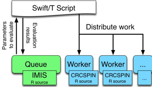
Figure 1: Overall relationship between IMIS and CRC-SPIN within the EMEWS framework.
